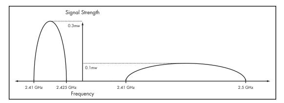
Figure 1.3: Conventional and DSSS radio signals
