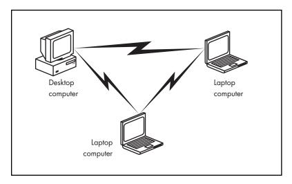
Figure 1.6: An ad hoc wireless network with three stations
